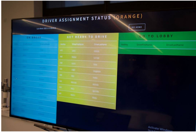
FIGURE 19 Driver Assignment Status board. The display is located in the drivers' break room and lets drivers know when they should get ready to drive, and when they should go to the operation center lobby.
