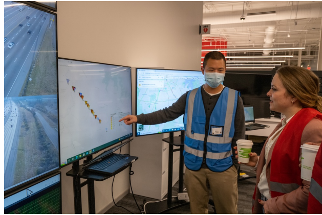
FIGURE 20 Vehicle Tracker System (middle screen). Co-author Jonathan Lee introduces the display to US DOE stakeholder, Heather Croteau. Located in the operation center, the realtime location, speed, direction, and control status of all deployed vehicles on the map.
