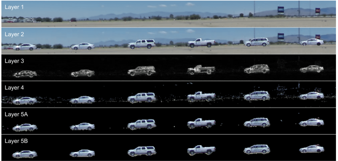
Fig. 2. Step-by-step visualization of background subtraction methods. Layer 1 shows a section of the estimated background within the first 15-s time interval in Experiment A. Layer 2 is the first frame of that time interval. Layer 3 is the square distance between layer 1 and layer 2. Layer 4 is the remaining foreground after removing pixels at locations that have square distance under 14. Layer 5A is the refined foreground after applying morphological transformation on layer 4. Layer 5B is the refined foreground after removing noise pixels outside the alpha complex of every vehicle from layer 4.
