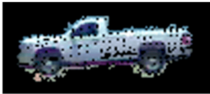
(a) Estimated vehicle template using DBSCAN, with holes due to errors in the background subtraction step.
